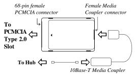
**Figure 1-B** Adapter with 10Base-2/10Base-T Coupler
